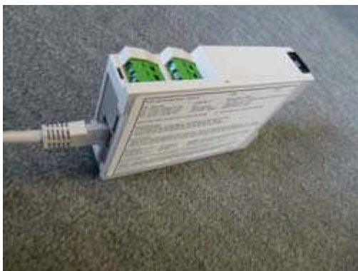
iBOX-2S module with 2 B micro SD card
